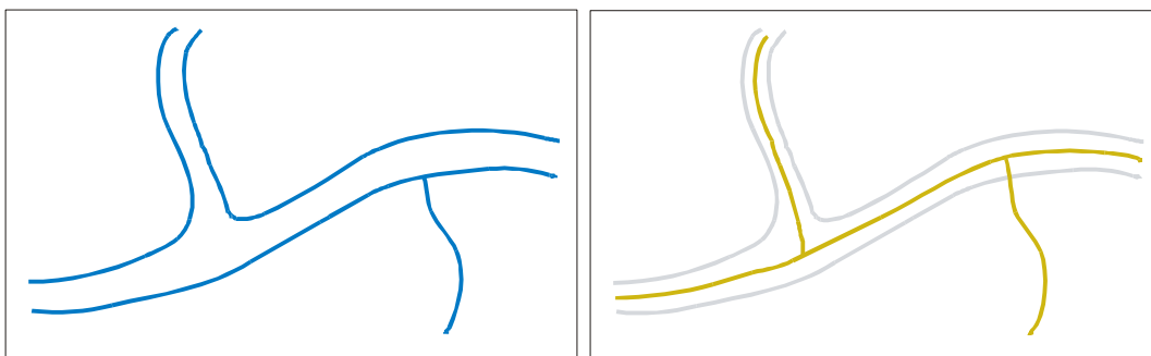
Figure 13 Left a line object before the parallel extraction and on the right after the parallels have been detected.
